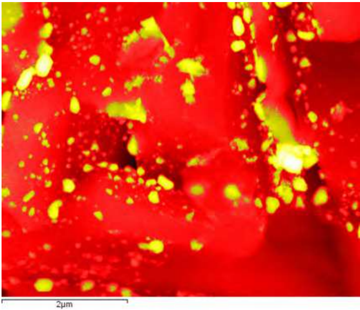
Fig. 13. Color rendering of a BSE image. The yellow areas represent Ag deposits. The red colored areas show the matrix ( \text{Al}_2\text{O}_3 ).
