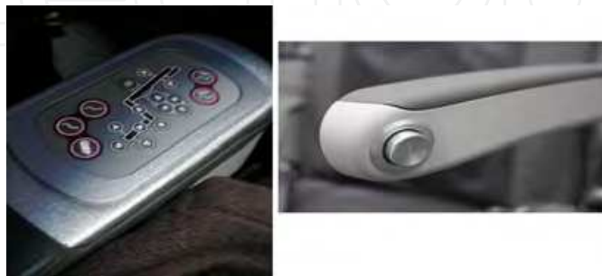
Fig. 3. Electronic Vs Mechanical seat adjustment
