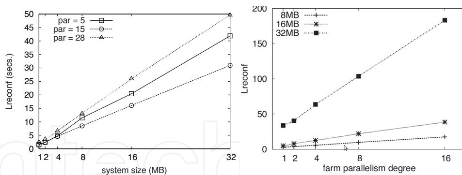
Fig. 6.  $L_{reconf}$  for the rollforward (left) and the rollback (right) switching from a source version (a task-farm) to a target version (a data-parallel) of the Solver ParMod. For the rollforward protocol  $L_{reconf}$  is dominated by the time spent for completing all the pending tasks in the source version, before starting the target one. For the rollback protocol  $L_{reconf}$  indicates the time necessary for re-executing all the rolled-back tasks.
