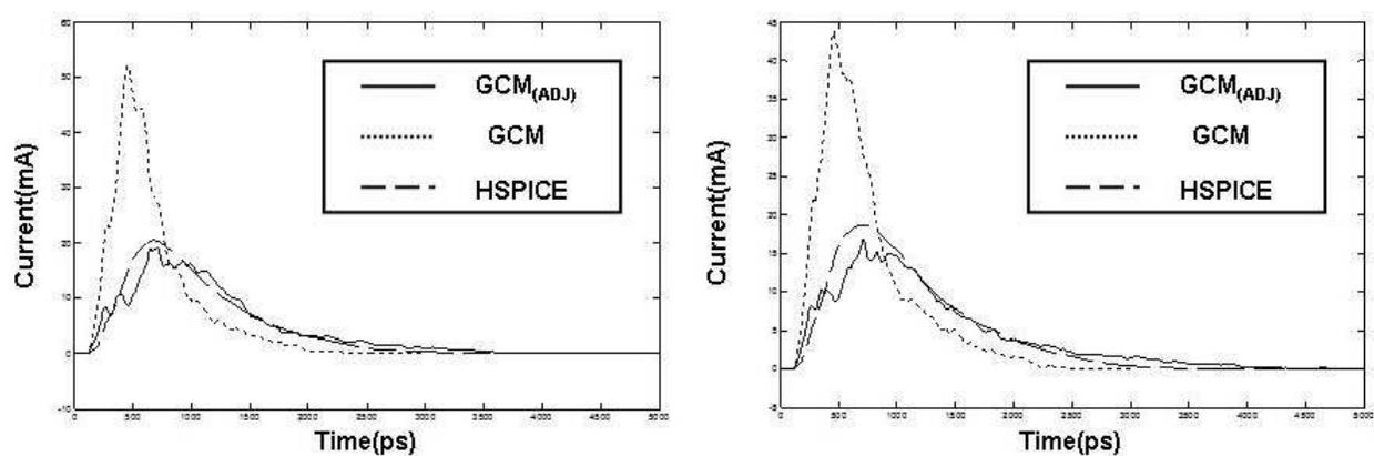
Fig. 24. The estimation supply current waveforms of c7552 with  $R_{WIRE}=10\text{ohm}$
