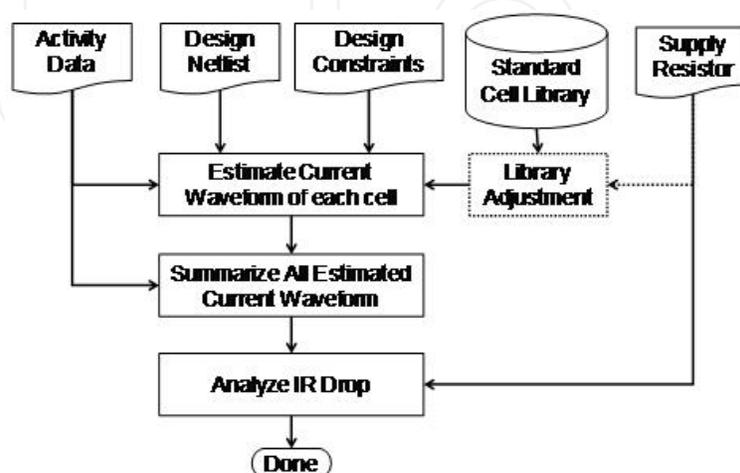
Fig. 3. The proposed gate-level IR-drop analysis flow
