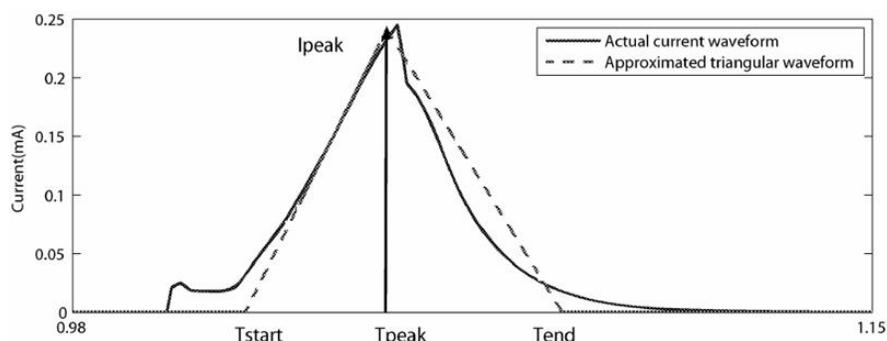
Fig. 4. The definition of the triangular current waveform
