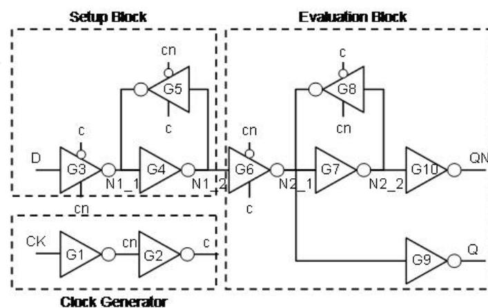
Fig. 12. The architecture of a typical DFF
