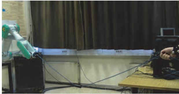
Fig. 14. Experimental setup for cooperative human-robot rope turning.
