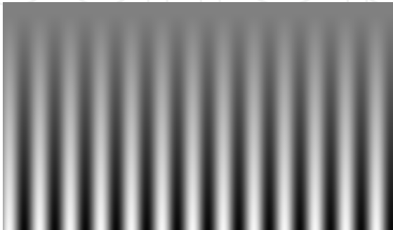
Fig. 3. Example of sinusoidal grating stimulus. Along the vertical axis of the screen, contrast becomes the highest in the bottom and lowest in the top of the pattern.
