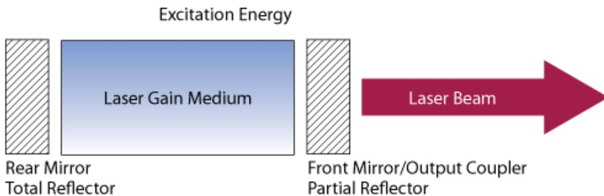
Fig. 1. The component parts of a typical laser
