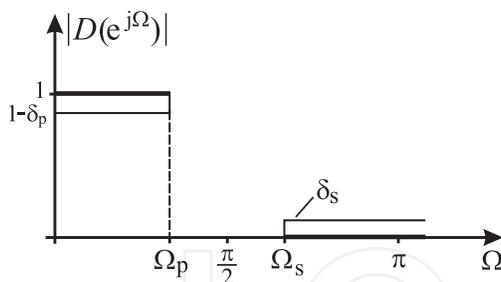
Fig. 8. Magnitude specification of minimum-phase IIR lowpass HBF;
