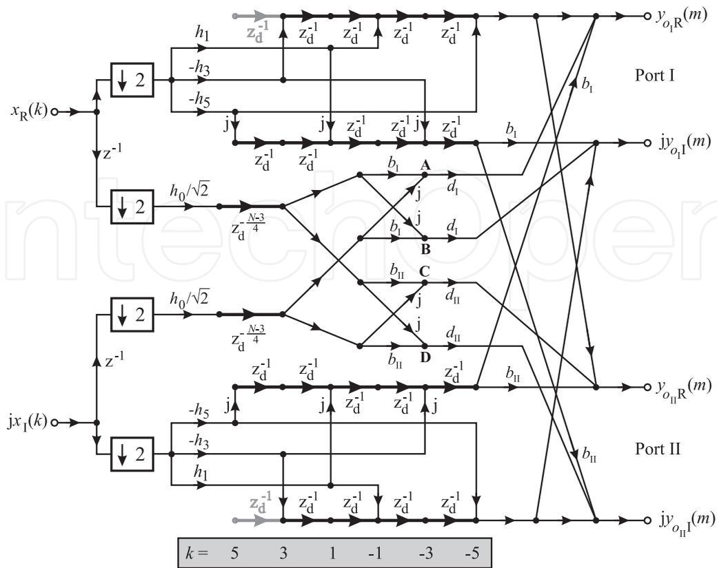
Fig. 24. COHBF approach to demultiplexing DF implementation with selectable transfer functions;  $N = 11$ ,  $b_i = (-1)^{o_i}$ ,  $d_i = (-1)^{\lfloor o_i/2 \rfloor}$ ;  $o_i \in \{0, 1, 2, 3\}$ ,  $i \in \{I, II\}$
