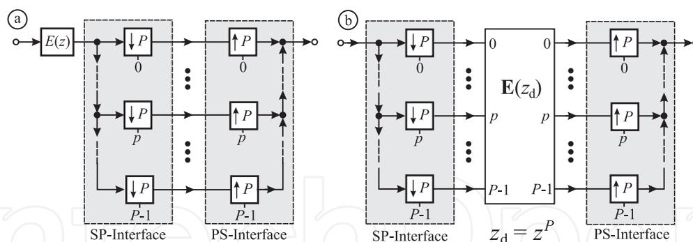
Fig. 29.  $P$ -Parallelisation of SISO subsystem  $E(z)$  to  $P \times P$  MIMO system  $\mathbf{E}(z_d)$
