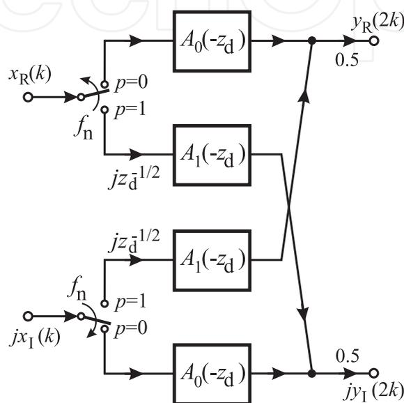
Fig. 15. Block structure of decimating minimum-phase IIR CHBF
