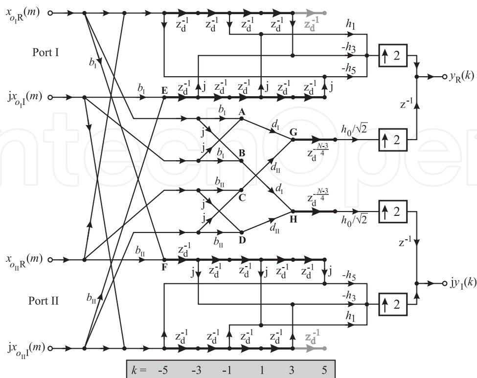
Fig. 26. COHBF approach to *multiplexing* DF implementation with selectable transfer functions derived by transposition from corresponding separating DF;  $N = 11$ ,  $b_i = (-1)^{o_i}$ ,  $d_i = (-1)^{\lfloor o_i/2 \rfloor}$ ;  $o_i \in \{0, 1, 2, 3\}$ ,  $i \in \{I, II\}$
