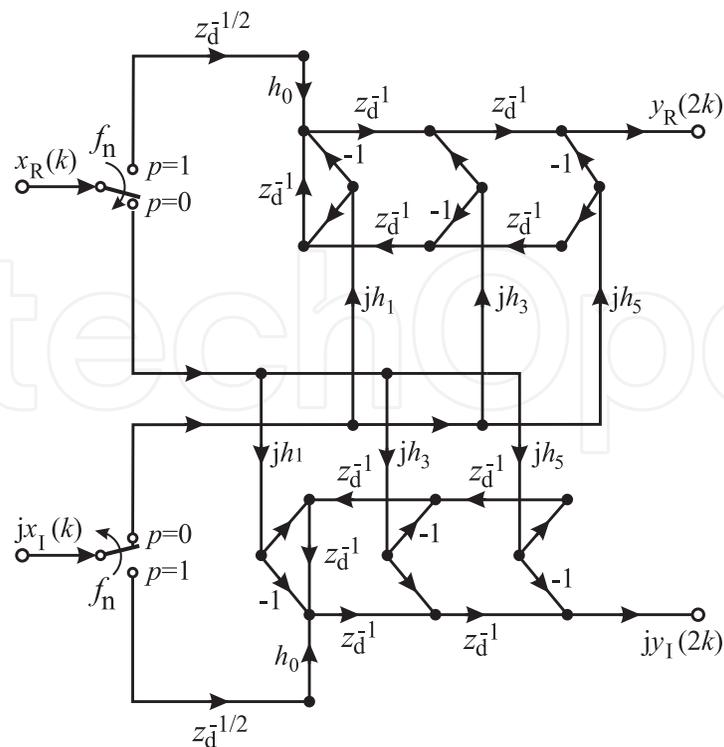
Fig. 13. Optimum SFG of decimating linear-phase FIR CHBF
