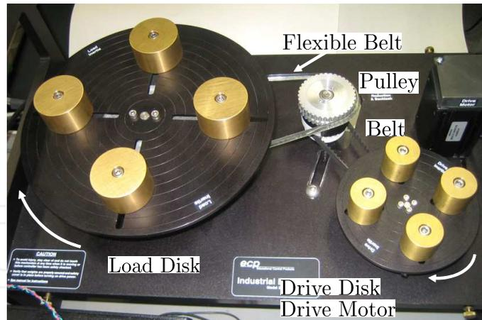
Fig. 6. Experimental set-up of a belt-driven two-mass system.
