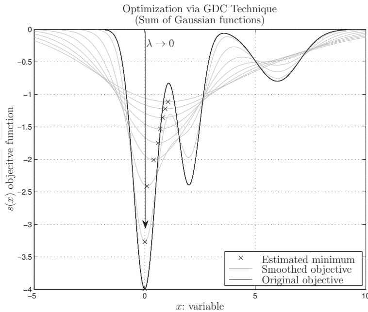
Fig. 4. Illustration of the GDC method. Starting from the original objective (dark line) and give a set of smoothing parameters  $\lambda$ , smoothed versions (thin line) of the original objective are computed. Iterating the process smooth-minimize-continue, the global optimum of the original objective can be found with high probability when the last minimization with  $\lambda = 0$  is performed.
