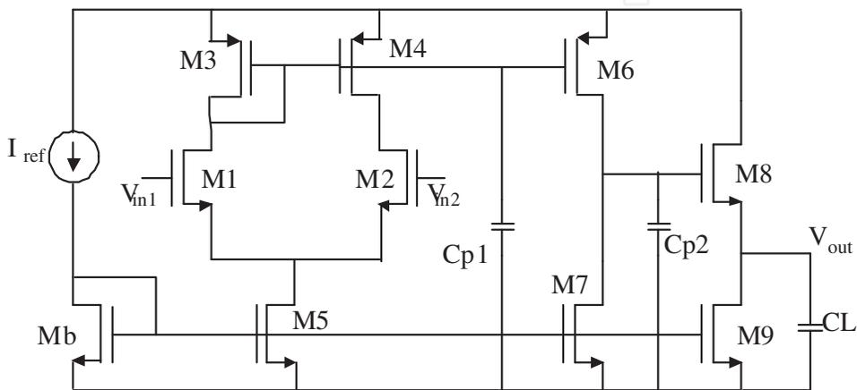
Fig. 3. Three stages uncompensated low voltage amplifier.
