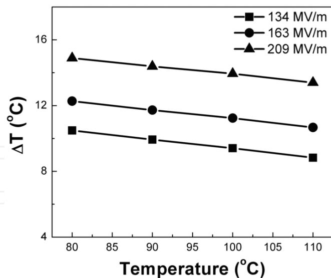
Fig. 12. ECE temperature changes versus temperature for 55/45 copolymer.
