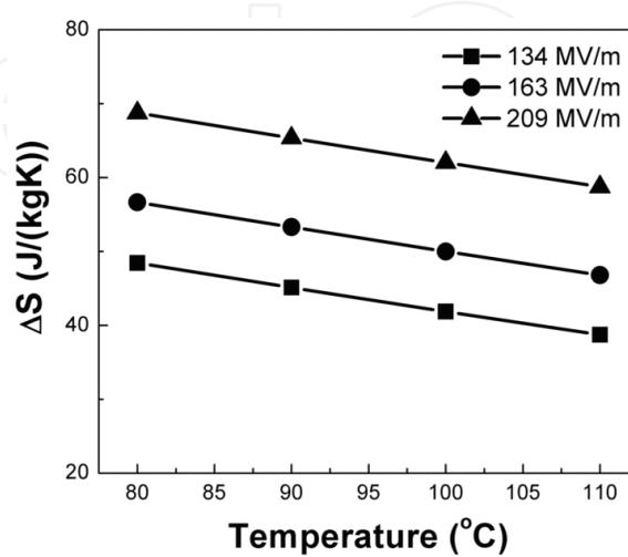
Fig. 11. ECE entropy changes versus temperature for 55/45 copolymer.
