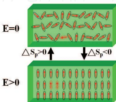
Fig. 1. Schematic drawing of the ECE process in a dipolar material. When  $E=0$ , the dipoles orient randomly. When  $E>0$ , especially larger than the coercive electric field, the dipoles orient along the electric field direction.
