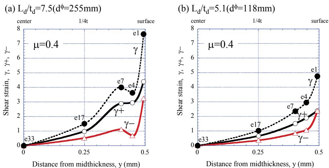
Fig. 10. Variations of the total shear strain  $\gamma$ , positive shear strain  $\gamma^+$ , and reverse shear strain  $\gamma^-$  through sheet thickness after rolling with  $\mu=0.4$ . Here, e1, e4, e7, e17 and e33 are displayed in the inset of Fig. 9.
