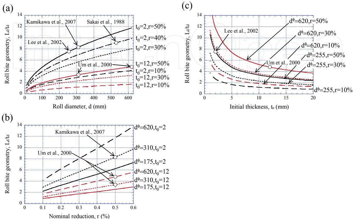
Fig. 16. Variations of the roll bite geometry  $L_d/t_d$  with (a) roll diameter  $d^\phi$ , (b) nominal reduction  $r$ , and (c) initial thickness  $t_0$ . Here, the open symbols indicate the rolling conditions employed in the literature.
