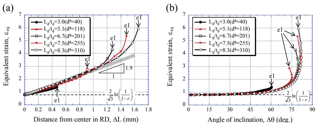
Fig. 13. Variations of  $\varepsilon_{eq}$  with (a)  $\Delta L$  and (b)  $\Delta\theta$  through thickness in 50% rolled Al with  $\mu=0.4$  under various  $L_d/t_d$  (Nos. 1-5 in Table 1). Here, e1 denotes data at the surface shown in the inset of Fig. 9.
