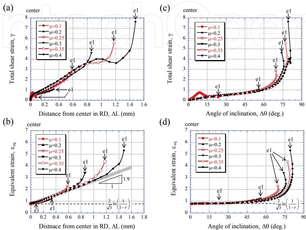
Fig. 12. Variations of (a)  $\gamma$  and (b)  $\varepsilon_{eq}$  with  $\Delta L$  and (c)  $\gamma$  and (d)  $\varepsilon_{eq}$  with  $\Delta\theta$  through thickness in 50% rolled Al for various friction coefficients  $\mu$  under  $L_d/t_d = 7.5$  (No. 2 in Table 1). Here, e1 denotes data at the sheet surface shown in the inset of Fig. 9.
