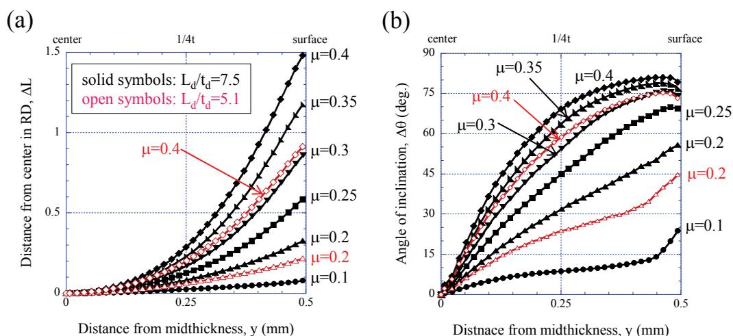
Fig. 8. Variations of (a)  $\Delta L$  and (b)  $\Delta\theta$  through sheet thickness after rolling with friction coefficient  $\mu$  under  $L_d/t_d = 7.5$  (No. 2 in Table 1) and  $L_d/t_d = 5.1$  (No. 4 in Table 1).
