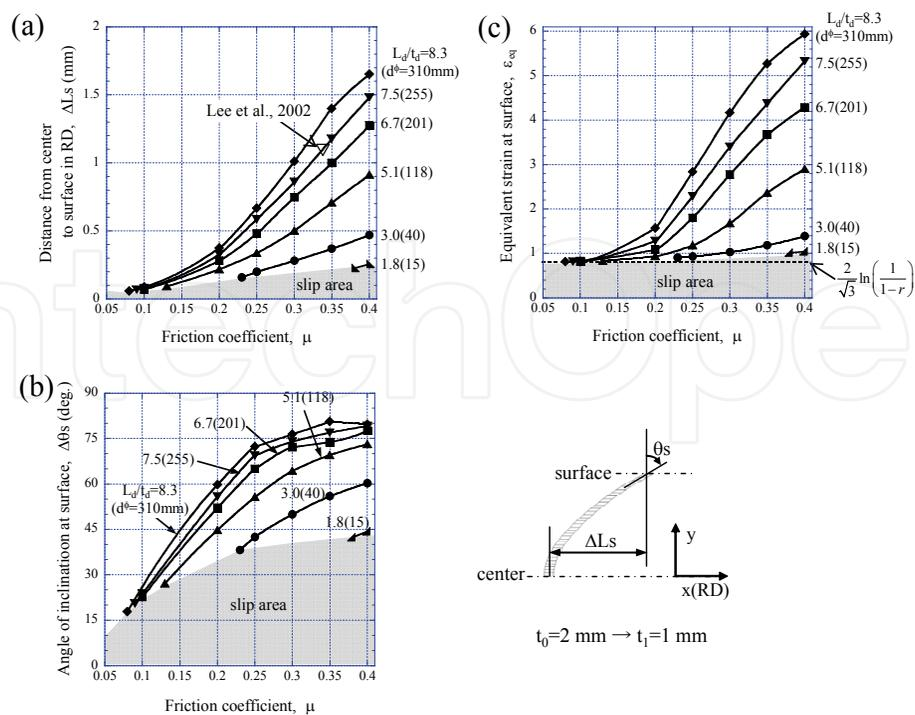
Fig. 6. (a)  $\Delta L_s$ , (b)  $\Delta\theta_s$ , and (c)  $\epsilon_{eq}$  at the surface of a 50% rolled Al sheet against  $\mu$  under different roll bite geometries  $L_d/t_d$  (Nos.1-6 shown in Table 1).
