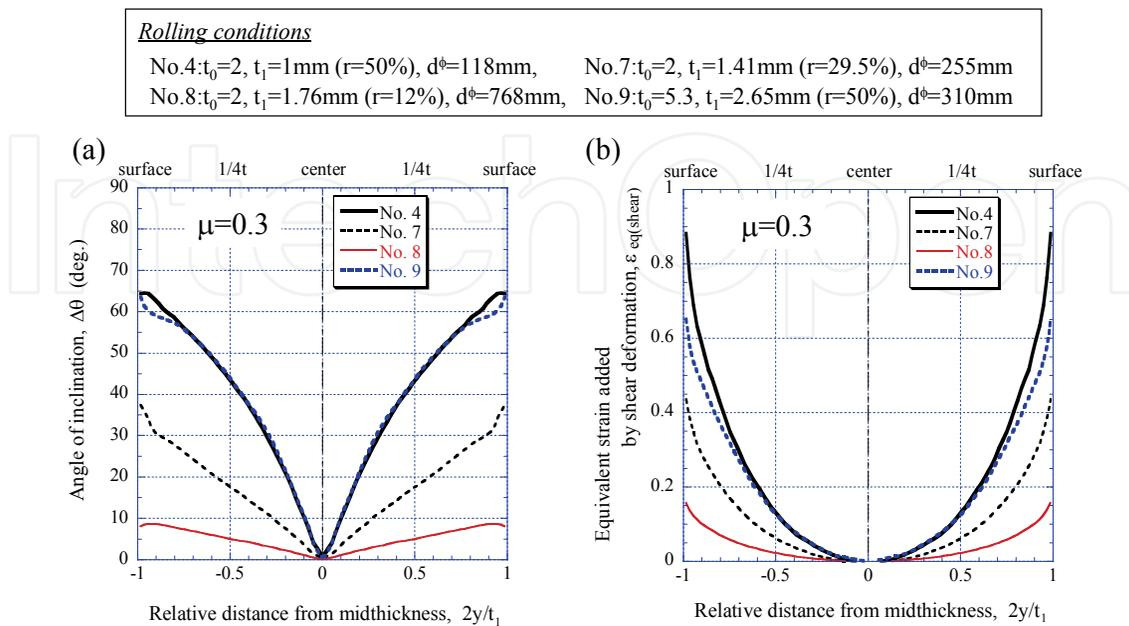
Fig. 14. Distributions of (a)  $\Delta\theta$  and (b) equivalent strain added by shear deformation,  $\varepsilon_{eq(shear)}$ , through sheet thickness in rolled Al with  $\mu=0.3$  under  $L_d/t_d=5.1$ . Here, full details of the rolling conditions are shown in Table 1.
