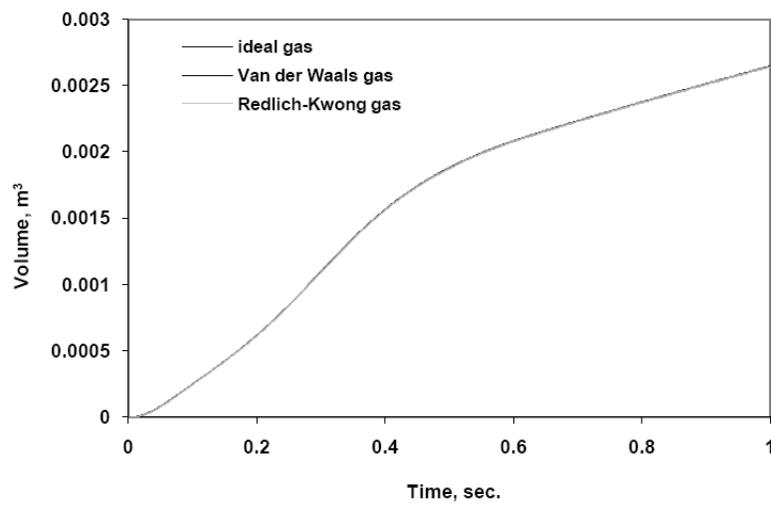
Fig. 3. Bubble volume *vs* times,  $h_0=1.5$  mm
