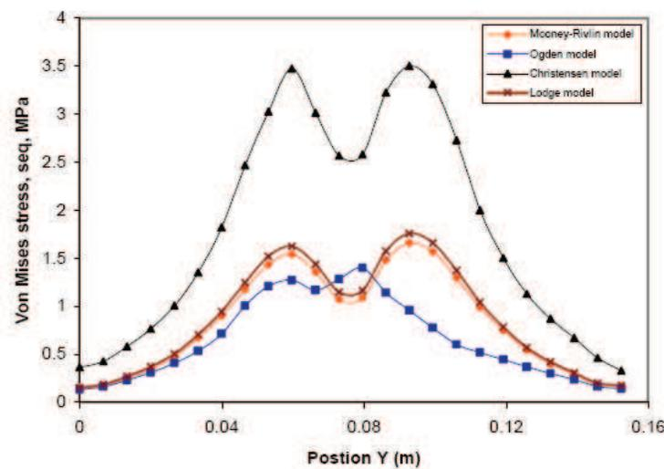
Fig. 11. Von Mises stress distribution, symmetry plan YZ
