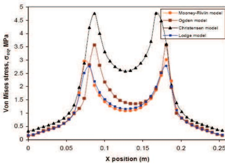
Fig. 10. Von Mises stress distribution, symmetry plan XZ
