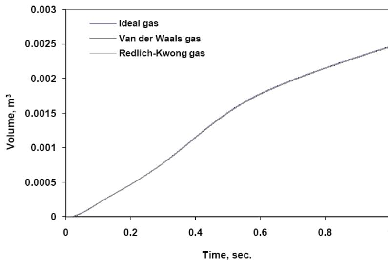
Fig. 5. Bubble volume *vs* times,  $h_0=3.0$  mm
