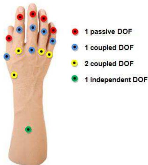
Fig. 7. Kinematic architecture of the proposed prosthesis
