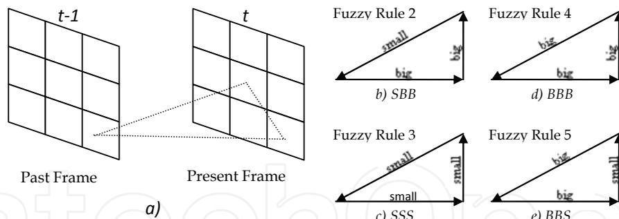
Fig. 1. Fuzzy Rules 2-5 in determination of the motion confidence in neighbouring frames. a) past and present Frames; b) Fuzzy Rule 2, *SBB*; c) Fuzzy Rule 3, *SSS*; d) Fuzzy Rule 4, *BBB*; e) Fuzzy Rule 5, *BBS*.
