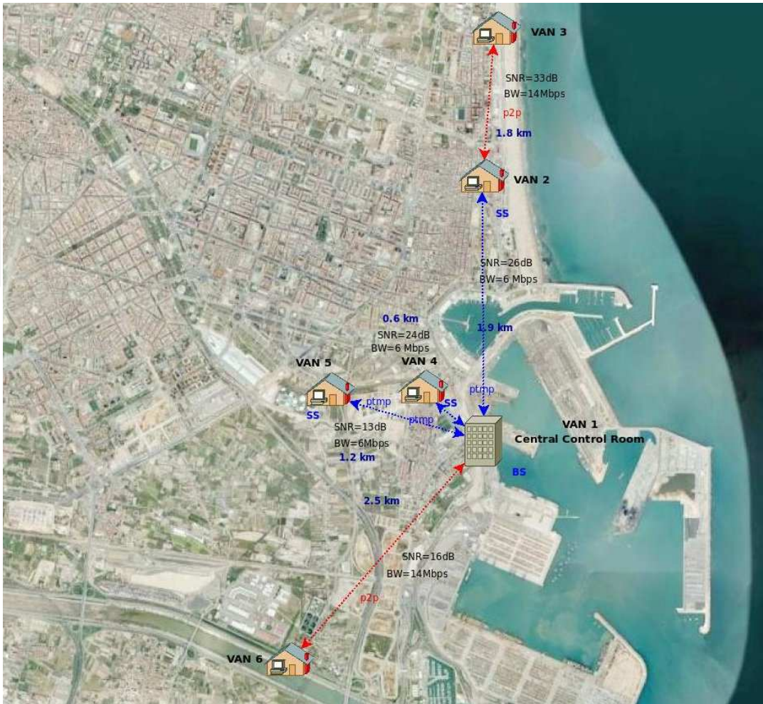
Fig. 4. WiMAX station distribution in a VAN control of utilities network application
