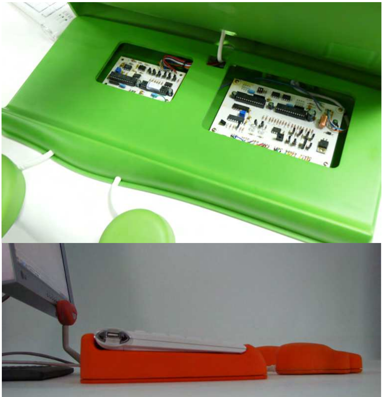
Fig. 10. Controller circuits underneath the keyboard base
