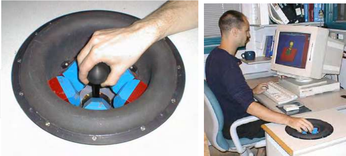
Fig. 3. Carnegie Mellon University Prototype (a) Levitated Handle Grasped by User, (b) Interaction with Simulated Environment
