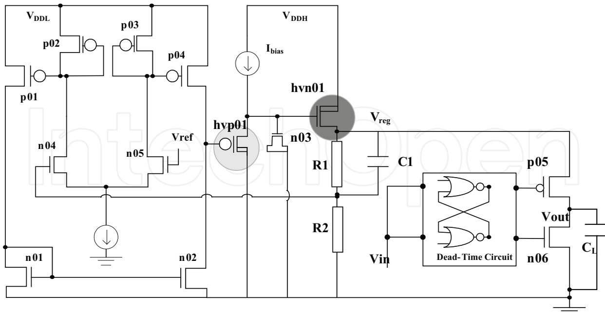
Fig. 2. Detail schematic of the proposed driver
