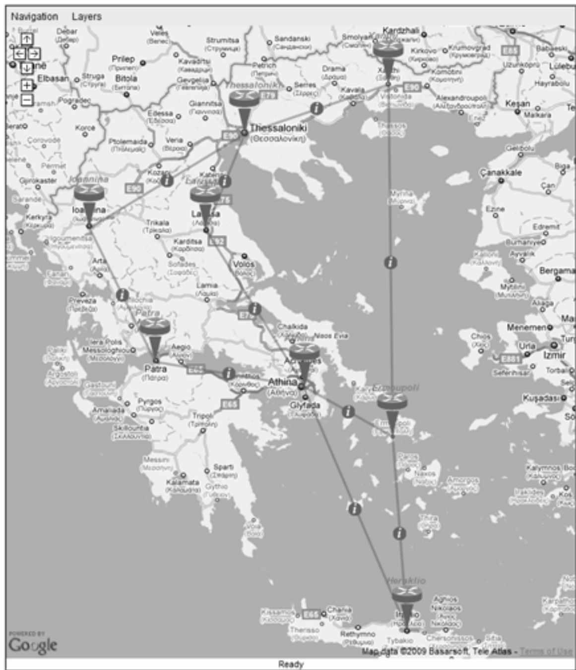
Fig. 1. GRNET’s Layer 3 Country Network Topology
