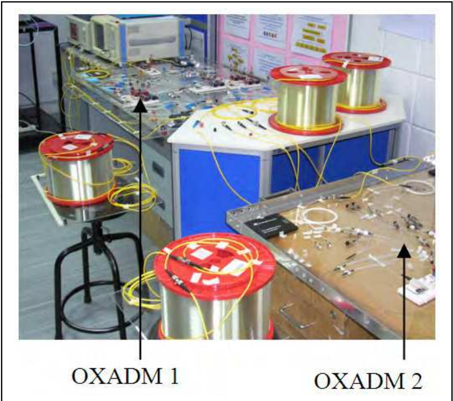
Fig. 28. Photographic view of two OXADM device prototypes set up in P2P network
