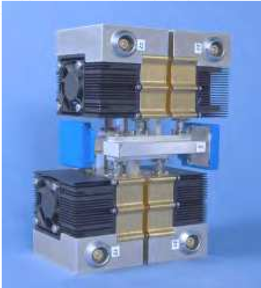
Fig. 7. Example of power amplifier using five-port distributed waveguide power splitter/combiner
