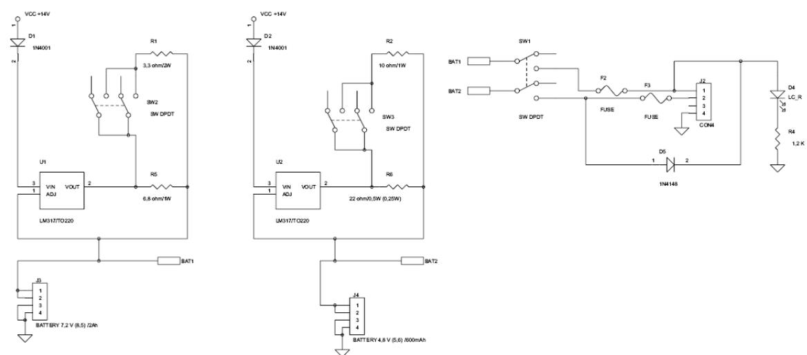
Fig. 13. Battery charger electronic scheme
