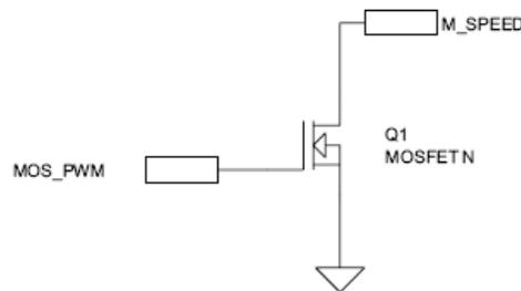
Fig. 8. Motor speed control
