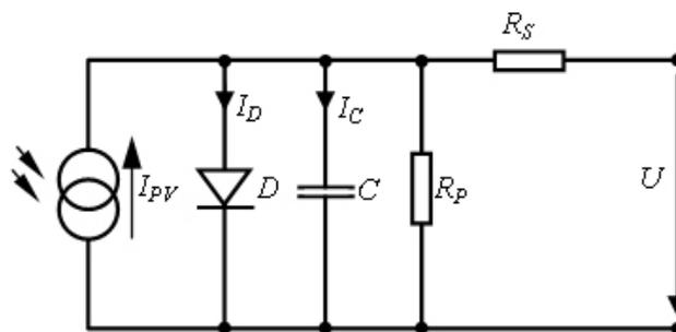
Fig. 1. Equivalent circuit diagram of a solar cell
