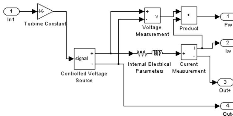
Fig. 7. Matlab-Simulink model of the generator
