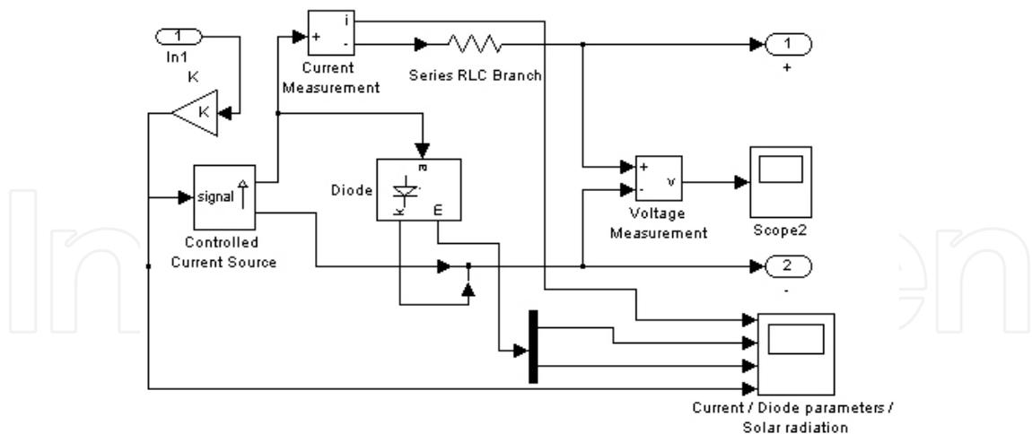
Fig. 3. Matlab Simulink implementation of the PV module.
