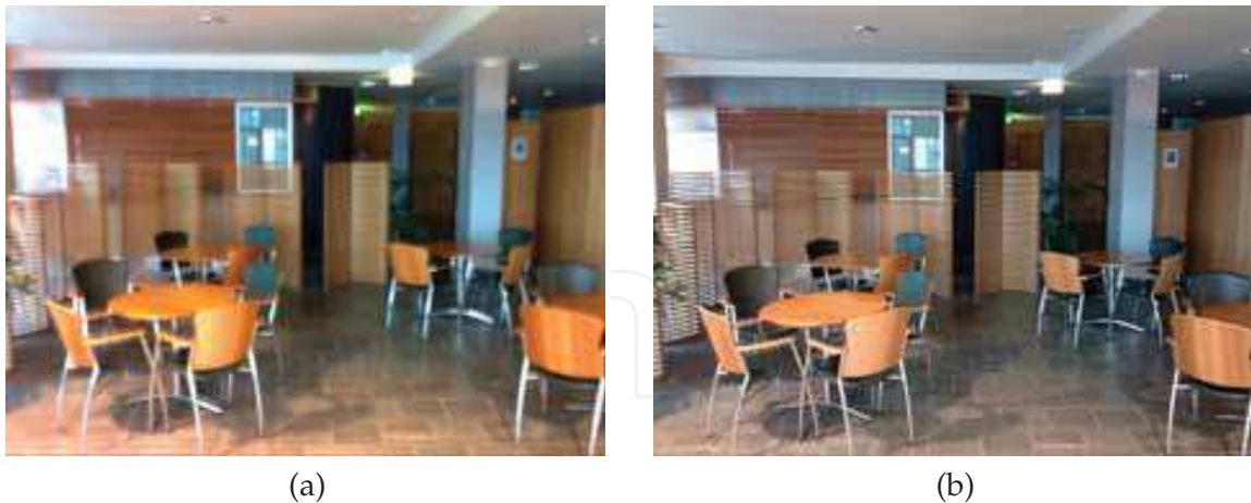
Fig. 6. Real imaging examples: (a) auto-exposed image taken with a camera phone (exposure time: 1.8 sec), (b) stabilized image by fusing four frames with exposure time of 0.3 sec each.
