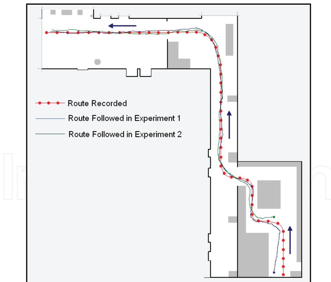
Figure 11. Route recorded by the leader robot and routes followed by a follower robot in two experiments with different initial point
