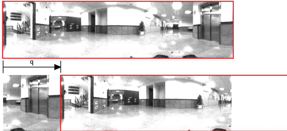
Figure 6. Two panoramic images taken in the same point but with different heading for the robot
