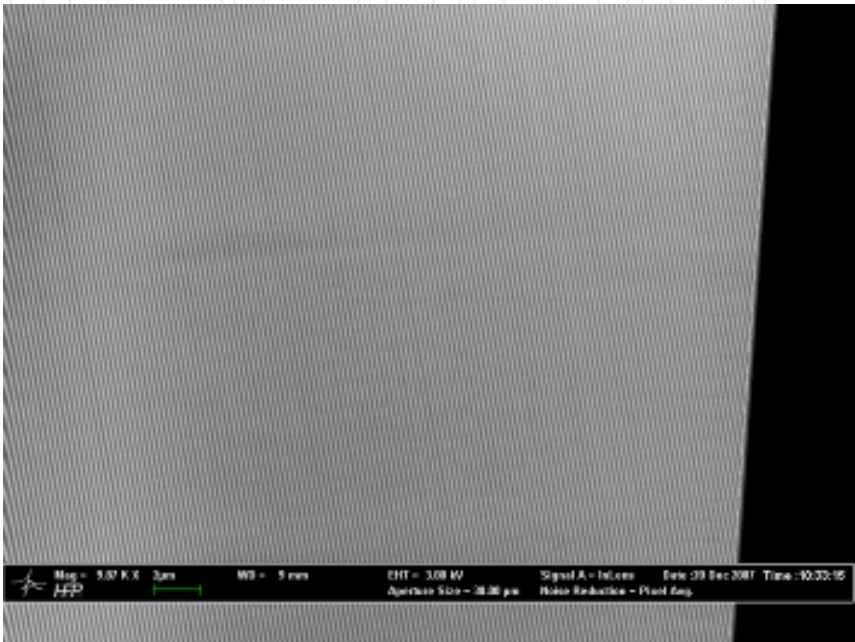
Fig. 22. SEM measurement of 50 nm half pitch imprinted data track features utilizing soft stamp imprint lithography
