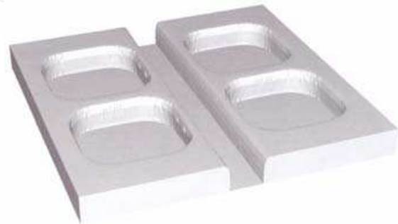
Fig. 20. Simulated 3D resist profiles for a layout consisting one 30 nm wide line and four 800 x 800 nm 2 squares at 50 keV e-beam
