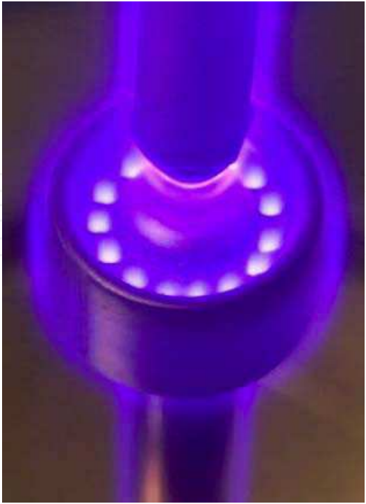
Fig. 2. Glow discharge and detailed view of the lower electrode.
