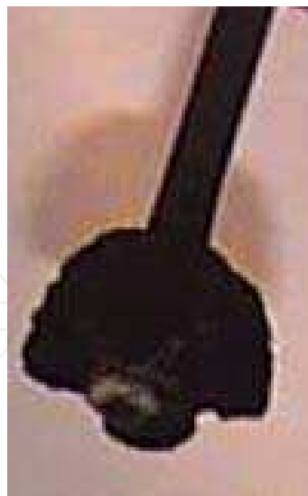
Fig. 6. Carbonaceous depot in cathode, when dc current is used
