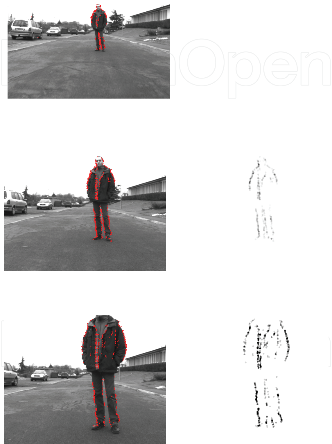
Figure 9. Warning values in different situations. Left column: flies are represented as dots. Right column: flies appear as spots as dark as their warning value is high
