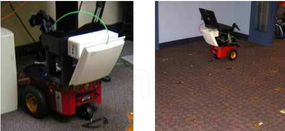
Fig. 11. Experimental setup. The Alien Reader was mounted on the platform of a robot (left). The RFID tags were placed on the floor in a regular grid pattern (right).
