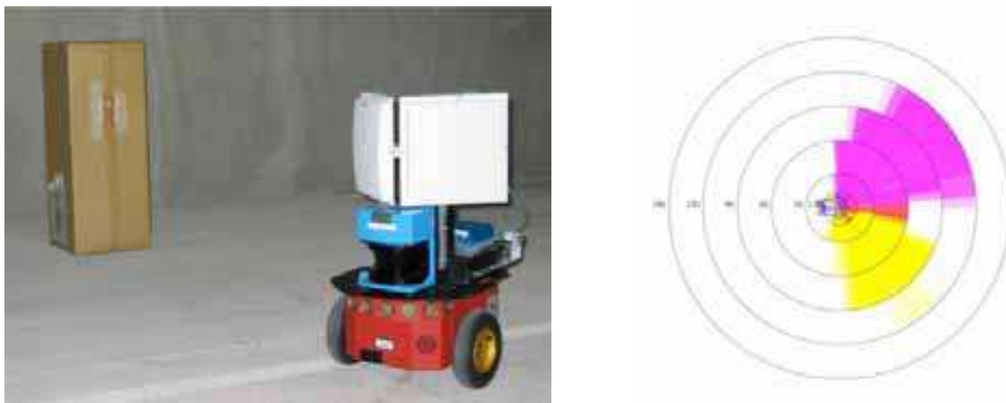
Fig. 9. This figure, adopted from (Hahnel, Burgard et al.), illustrates the experimental setup and learning a probabilistic sensor model for the RFID antenna.
