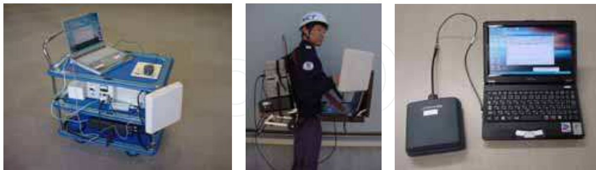
Fig. 2. RFID Writer/ Reader for Collection of Damage Information (Left: cart-mounted type, Center: backpack-mounted type; Right: handheld type)
