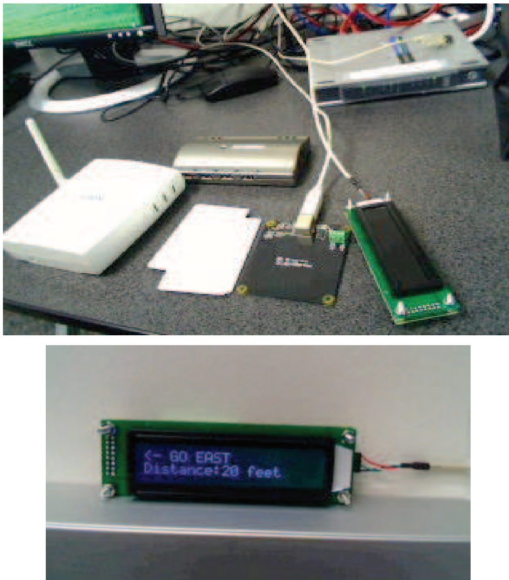
Fig. 2. Phidget RFID reader, EM4102 tags, USB servers, 20X2 PhidgetTextLCD
