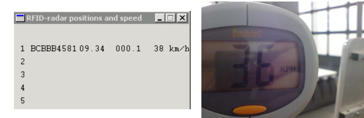
Fig. 17. Comparison between the speeds measured by the RFID system and a K-band radar
