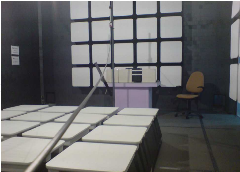
Fig. 15. View of experimental setup in the anechoic chamber for speed measurements
