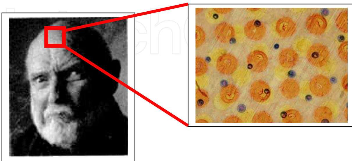
Fig. 10. A flexo printed bold face and its magnification.
