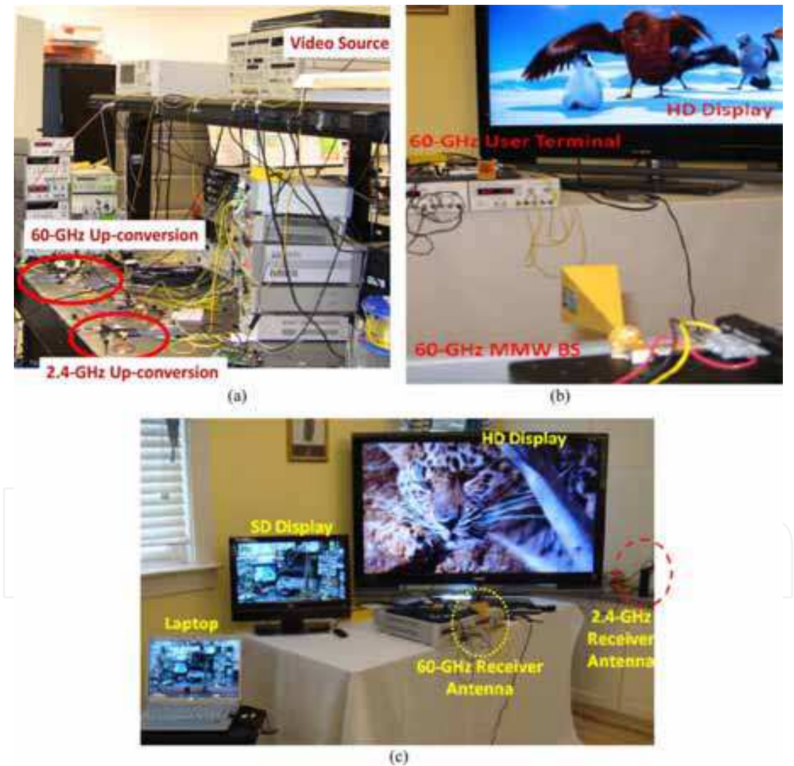
Fig. 39. Transmitter and receiver of the 3-screen, dual-service 2.4-GHz and 60-GHz RoF carrying 270-Mbps SD and 1.485-Gbps HD video content. (a) Transmitter at Centergy lab at 10th Street, (b) 60-GHz Wireless setup at residential lab at 5th Street, and (c) 3-screen receiver at residential lab.
