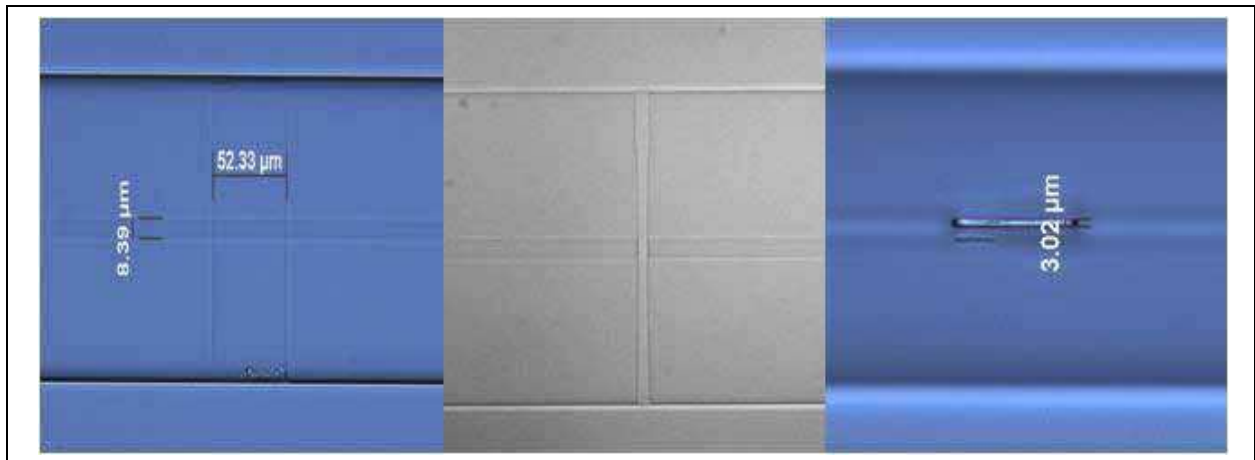
Fig. 8. Micro-channels fabricated in standard fibre using fs inscription and chemical etching (Y. Lai et al., 2006).
