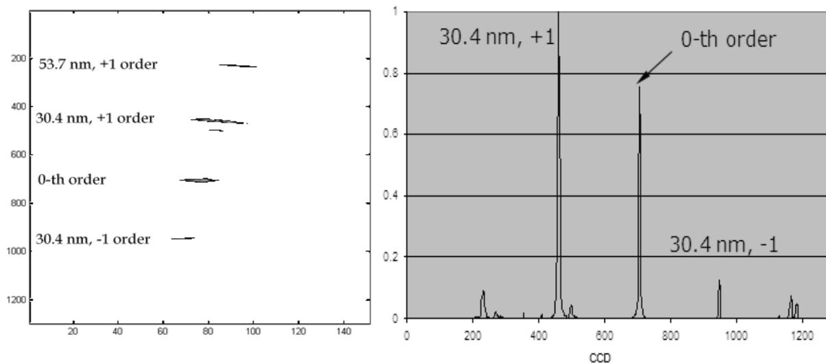
Fig. 11. Spectrum of He emissions from an hollow-cathode lamp, taken by a XUV-enhanced CCD detector placed in the output plane. Both gratings are operated in the condition  $\alpha = 0$ . A cross section along the CCD column num. 70 is shown on the right.
