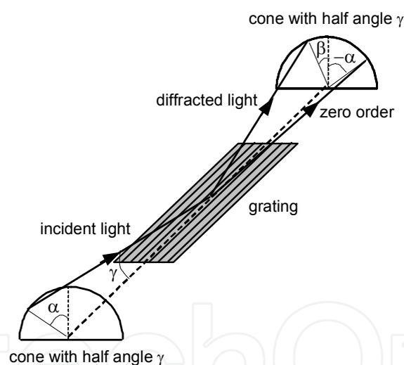
Fig. 3. The off-plane geometry.
