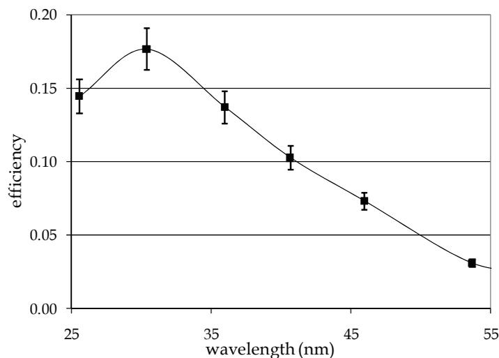
Fig. 13. Absolute efficiency of the TDC monochromator. Both gratings are operated in 1<sup>st</sup> diffraction order.
