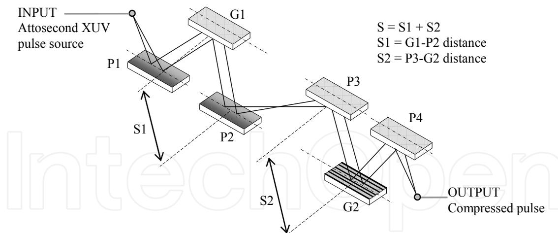
Fig. 16. Layout of the XUV attosecond compressor.
