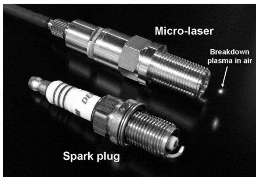
Fig. 15. Prototype spark plug size micro-laser head and a conventional spark plug
