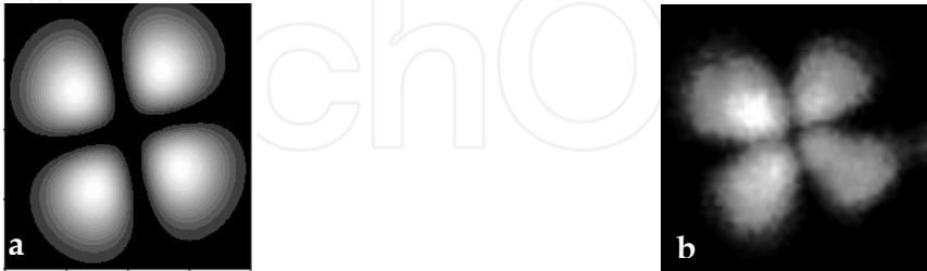
Fig. 3. Theoretical (a) and experimental (b) (Khazanov et al., 2000) intensity distributions of depolarized beam.
