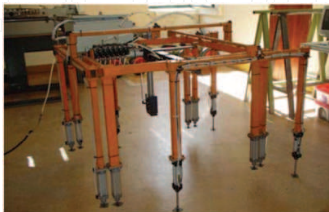
Fig. 10. The pneumatic version of the Poseidon robot
