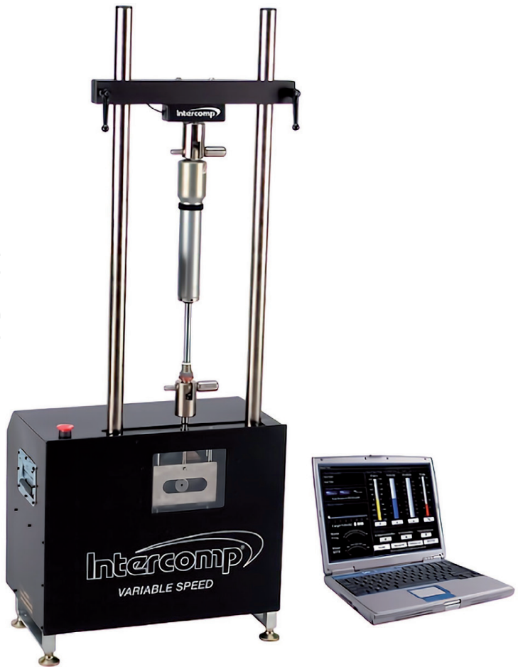
Figure 2. Intercomp 3HP shock dyno 1.0–55 in/s ($8895.00).
