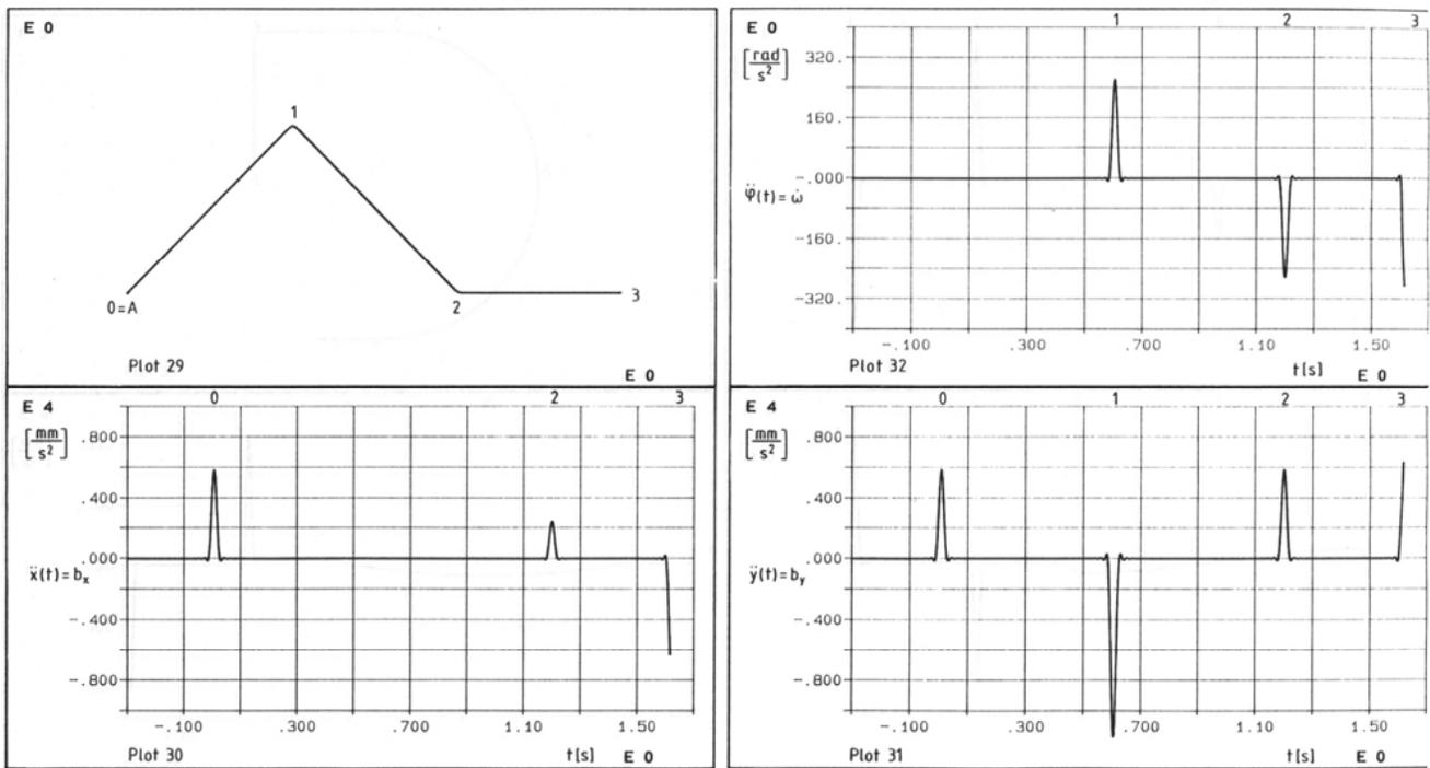
Figure 11. First part of the test trajectory and corresponding acceleration profiles
