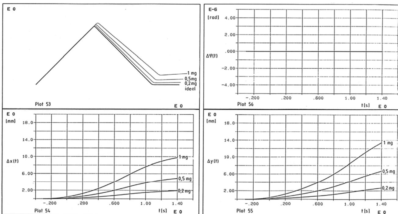
Figure 12. Overall measurement error due to bias errors
