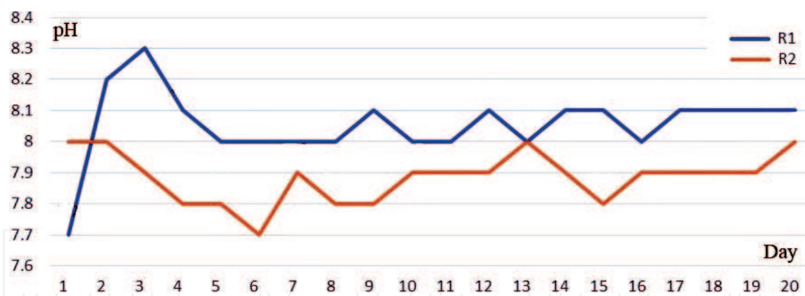
Figure 12. Substrate pH variation in time, first batch on 4 L reactors.
