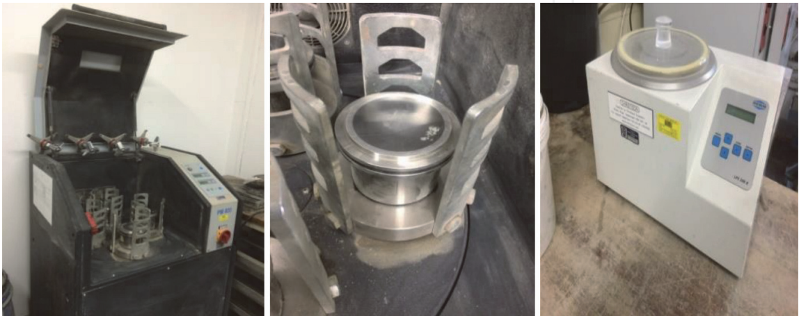
Figure 1. Laboratory grinder and air-jet sieve for collecting ground PC clinker.
