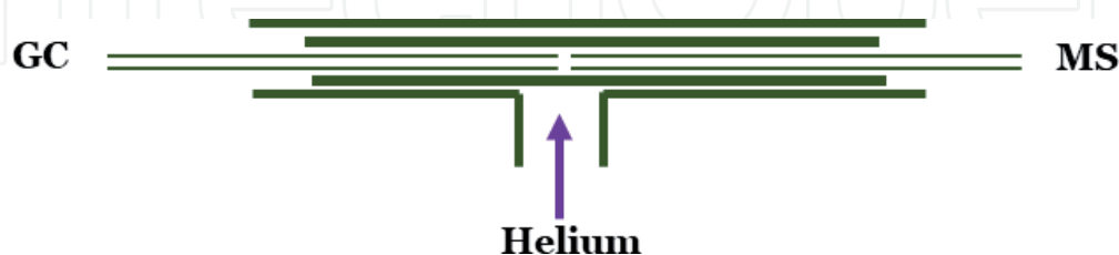
Figure 2. Schematic representation of an open-coupling system.
