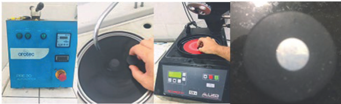
Figure 9. Mounting, sanding, polishing, and finished sample.
