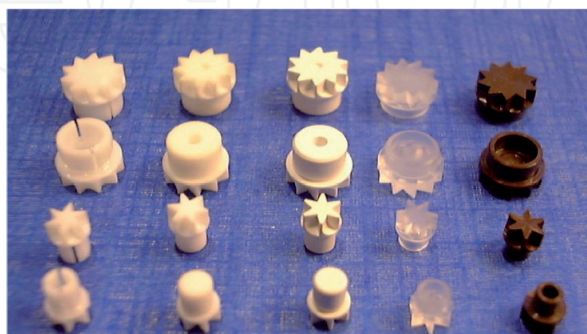
Figure 8. Type of caps used for rotors (typical materials used \text{ZrO}_2 , Macor, KeI and Vespel) [40].
