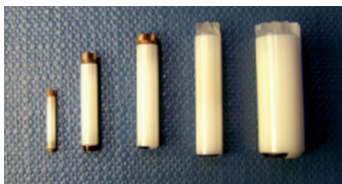
Figure 7. Rotors of different capacities are used for sample packing in ^{29}\text{Si} solid-state NMR [40].
