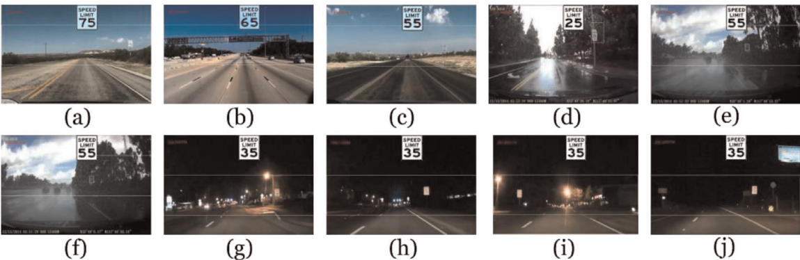
Figure 35. The overall results for rectangular speed limit signs detection (a-c) during the daytime (d) during the cloudy weather (e-f) during the rain (g-j) during the nighttime.
